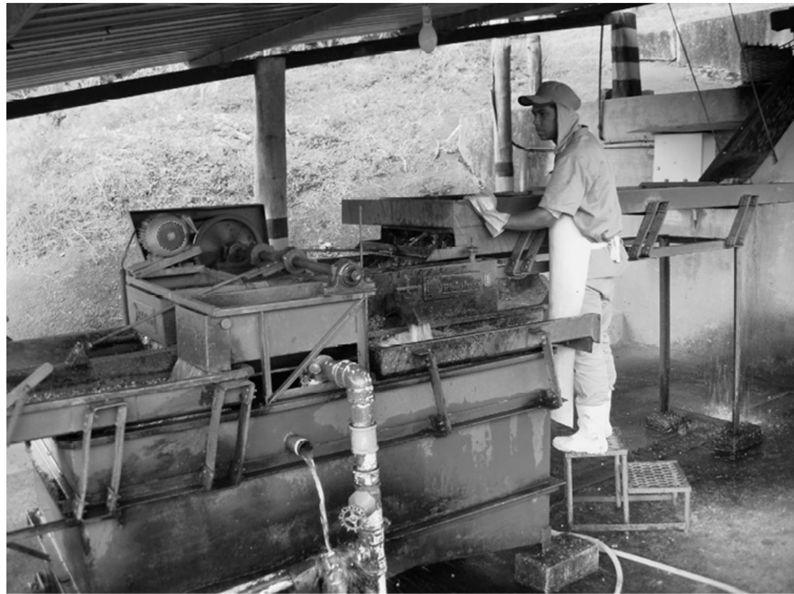
Figure 5.1. Depulping coffee on a mechanized farm, Sertãozinho in Sao Paulo State, Brazil. Few small coffee farmers possess this type of protective clothing. Photo by Robert Thurston.
